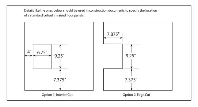
Sample Specification for the air-sealing grommet in Section 09 69 00
