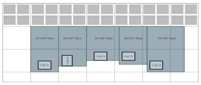
Tate has identified and offers a standard factory cut-out location that works with most imperial and metric sized racks and ensures that the cutout is always in the proper location inside the back door of the rack.
