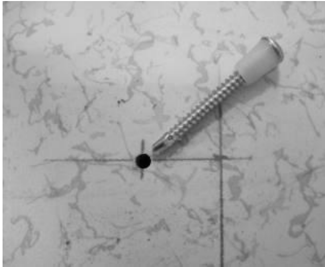
Figures 22 and 232: #6 x 1-1/4" screw and nylon spacer
