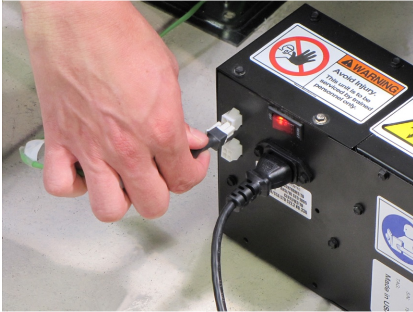
Figure 12 - Connecting LV Power feed to Power Module
