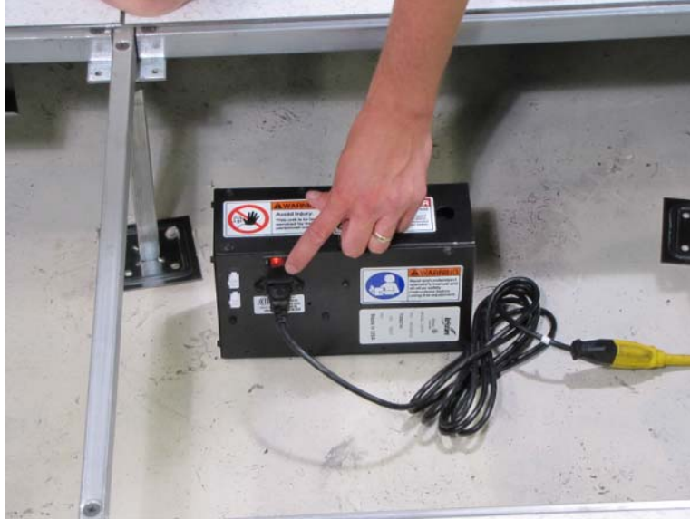
Figure 10 - Powering the Power Module On
